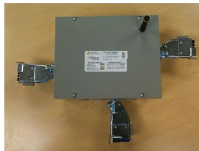
The Virticus Junction Box (VJB) controls 3 fixtures off one side and 3 off the other. The VJB was designed specifically to support an ease of installation and required no “wiring” of pieces - “plug in and go”.
